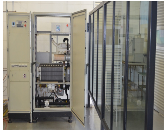
Figure 15. 5 kW PEMFC module constructed in collaboration with Electrocell using technology developed at IPEN.
