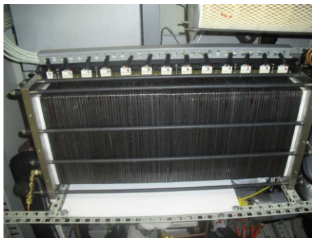
Figure 8. PEM fuel cell stack of 5 kW electric power, using technology developed at IPEN.
