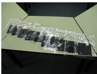
Figure 7. Membrane-Electrode-Assembly (MEA) with 250 cm 2 electrode area fabricated by sieve printing.
