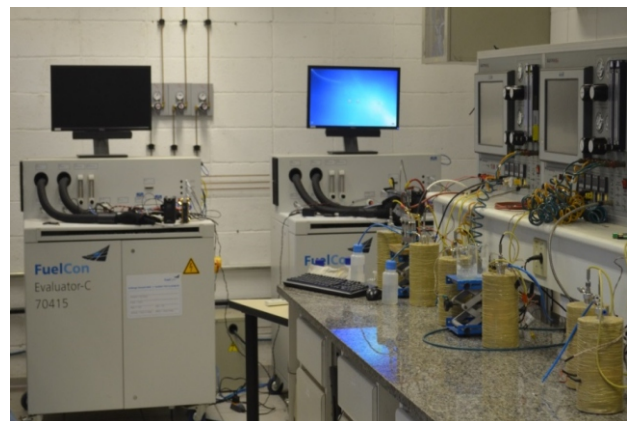
Figure 16. New test stations for PEMFC life cycle evaluation.
